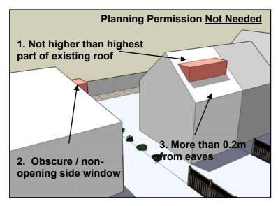
**Note:** For Building Regulations approval a fire escape window / opening window <u>is required</u> for each room within the roofspace when **on a bungalow**
