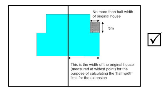
In the following example, although the extension is less than half the width of the original house and extends beyond the rear wall at 'A' by only three metres, it extends beyond the rear wall 'B' by more than three metres. It would therefore not be permitted development and will require an application for planning permission.
